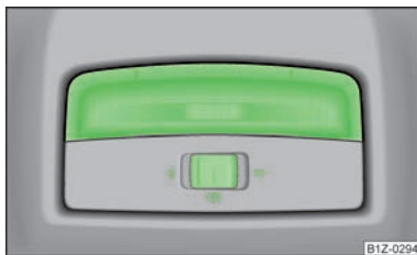
Fig. 30 Interior lighting - version 2
