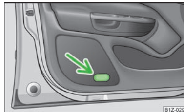
Fig. 31 Front door: Warning light
